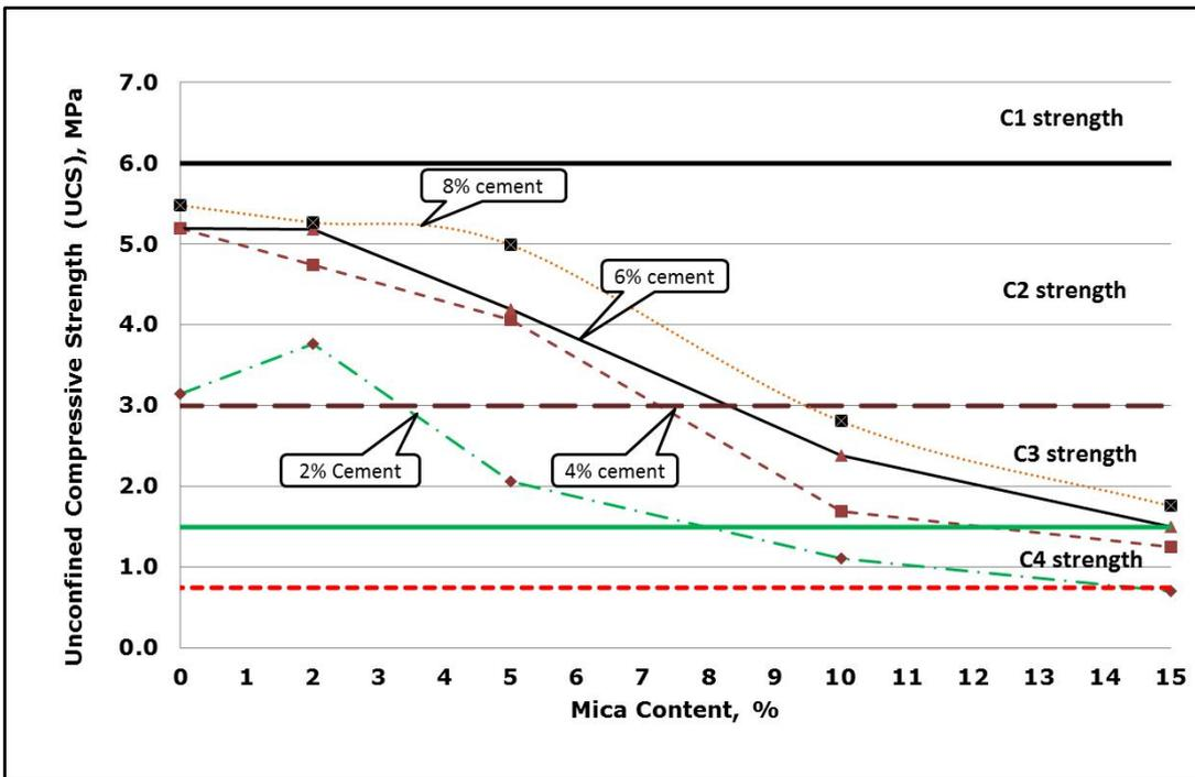
Figure 2: Influence of Mica in weathered granite on the UCS using cement as a stabilising agent (Mshali and Visser, 2012)
