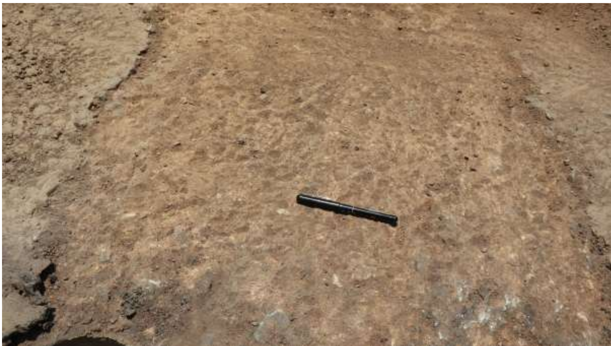
Photograph 7 Condition of the exposed base-layer at the end of the test after removal of the surfacing with a hammer and chisel
